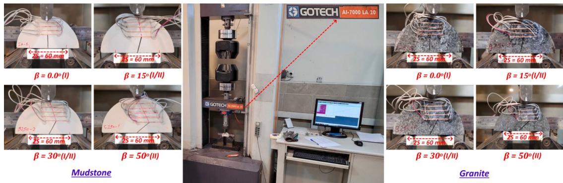
Fig. 5. Servo hydraulic machine used in this study with set up of three points bending test to obtain four different mode mixites in mudstone and granite samples.
