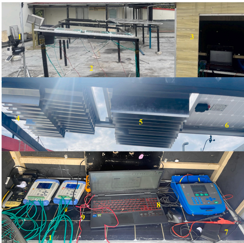
Fig. 5. A demonstration of the experimental rig in a way that 1) is Davis Vantage Pro2 weather station, 2) is the three modules, 3) is data collection house, 4) is the new heat sink, 5) is the heat sink with rectangular fin, 6) is PV alone, 7) is MP-11 I-V analyser, 8) is a computer, 9) is DT80 data logger, and 10) is K-type thermocouples.
