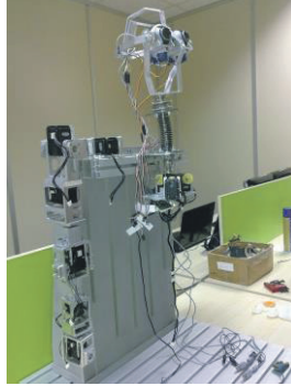
Figure 1. UMAY with 7 DOF head and 6DOF arm
