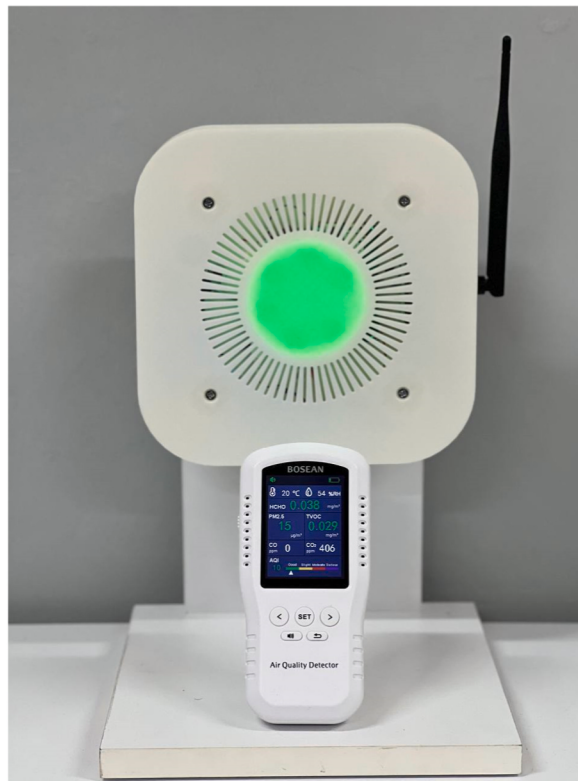
Fig. 3. Co-location of the developed IoT air-quality unit (back) and the BOSEAN T-Z01Pro reference device (front) during the calibration and validation experiment.
