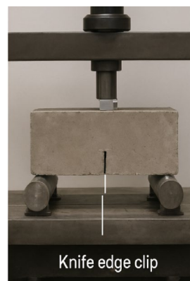
Fig. 3. Three-point bending test.
