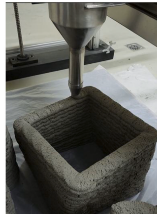
Fig. 20. Photos of the printing of large-scale elements using the developed 3DPC mixtures.
