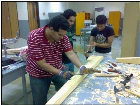
Figure 7b: Sample workshop activity of graving wood to manufacture the blades.
