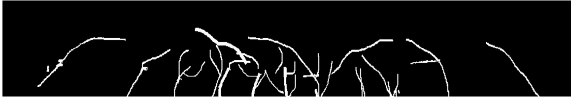
Figure 17. Image processing for cracks in BDCM (15-3) beams.
