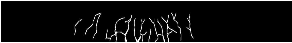
Figure 14. Image processing for cracks in BDCO (15-3) beams.
