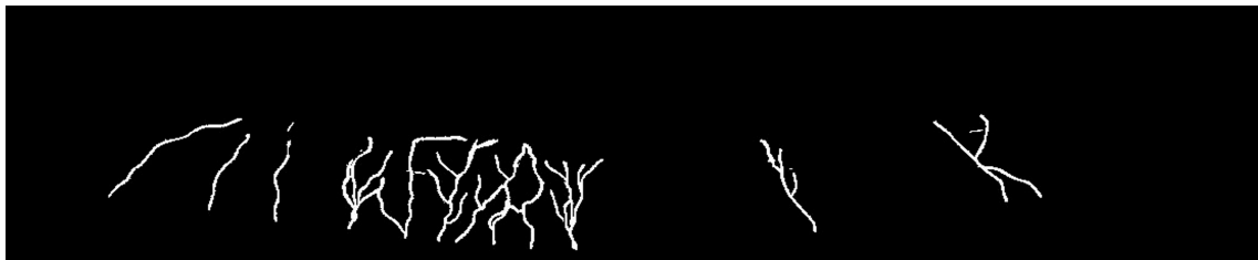
Figure 20. Image processing for cracks in BDCM (10-0.5) (15-1) beams.
