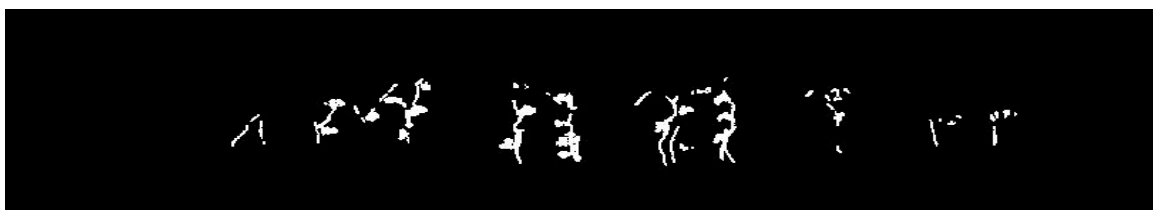
Figure 11. Image processing for cracks in SBDCM (15-1) beams.
