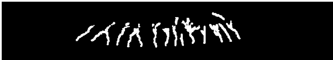
Figure 9. Image processing for cracks in BDCM (10-3) beams.
