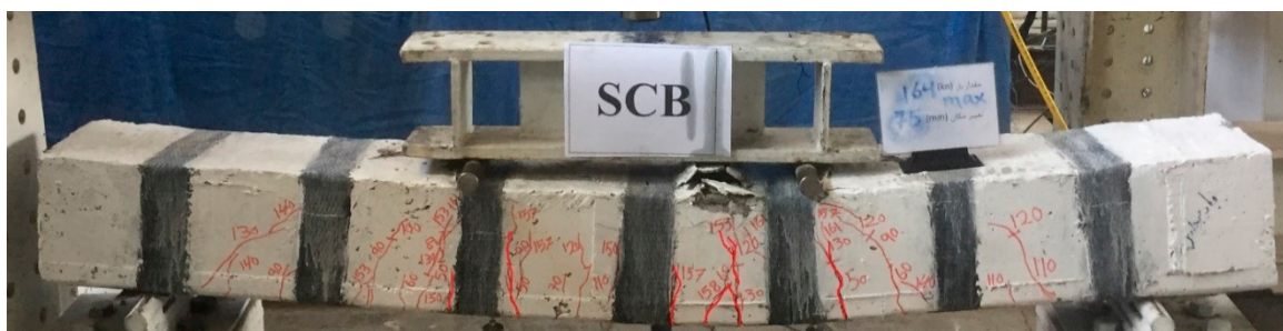
Figure 2. Depicting cracks to be subjected to image processing following beam failure.
