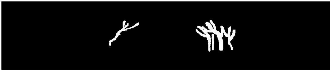
Figure 27. Image processing for cracks in BDRS beams.
