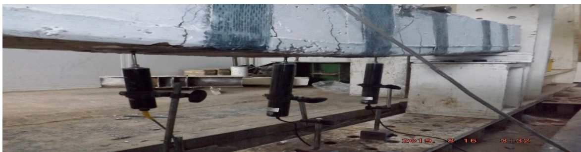
Figure 1. Recording of vertical changes in concrete beams.
