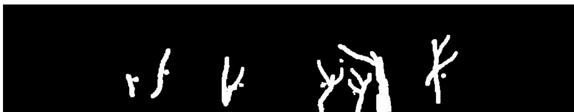
Figure 24. Image processing for cracks in SBDRA beams.
