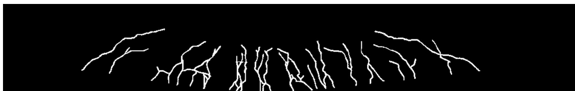
Figure 7. Image processing of cracks in CB beams.
