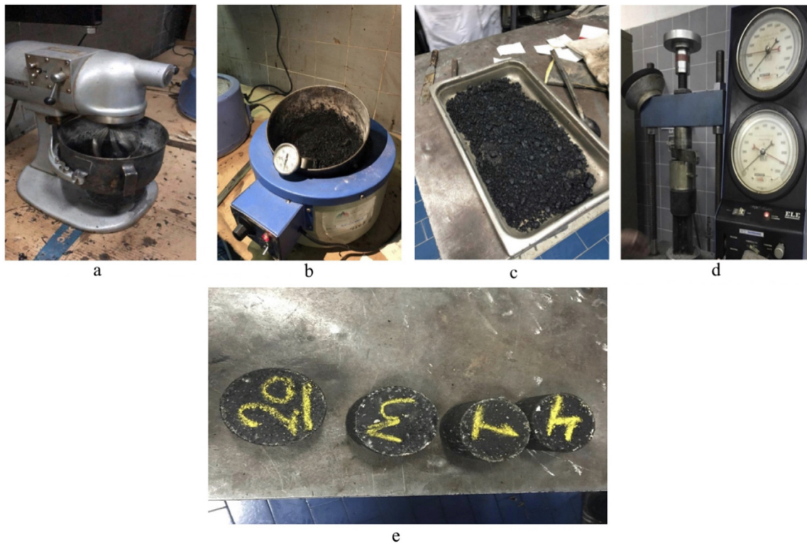
Fig. 5. Preparation of Asphalt-Concrete samples using Marshall.
