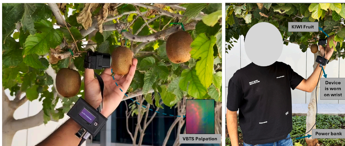
Fig. 10. On-tree demonstration of the wearable device for real-time kiwifruit firmness assessment. This figure shows the device in a field setting, estimating firmness directly on the tree using palpation-based sensing. The battery-powered, wrist-worn design supports portable, non-destructive use. The setup demonstrates on-tree feasibility.
