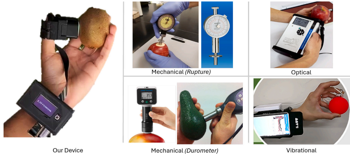
Fig. 9. Comparison of the proposed wearable device and traditional fruit firmness testers. The proposed device integrates human dexterity with AI-driven tactile sensing, enabling non-destructive, real-time firmness estimation. In contrast, conventional methods—including mechanical (rupture and durometer), optical, and vibrational techniques are often invasive or influenced by environmental factors, limiting their adaptability and accuracy.
