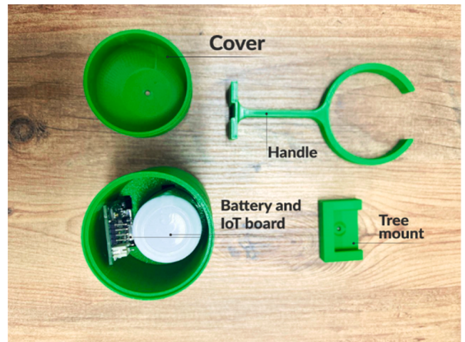
Fig. 4. Components of the IoT sound detection node.
