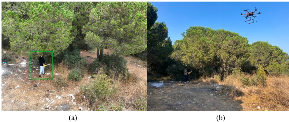
Fig. 17. Drone-captured image demonstrating human detection in a forested area: (a) image illustrating the detection of a human presence within the forest, (b) AI-powered drone arriving at the designated detection area.
