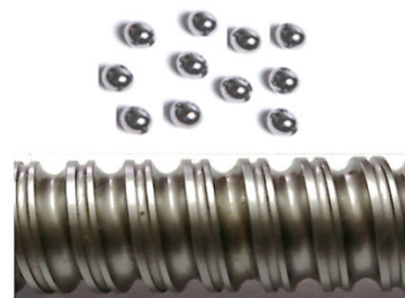
FIGURE 9. Mechanical backlash fault by changing recirculating balls size.
