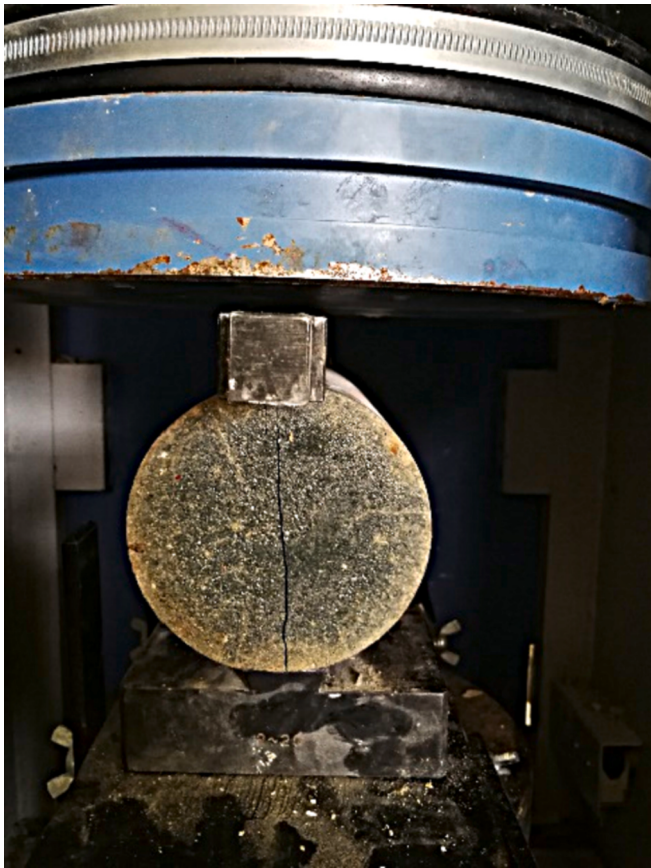
Fig. 1. Failure of 100 mm × 200 mm alkali-activated mortar samples during splitting tensile strength test.
