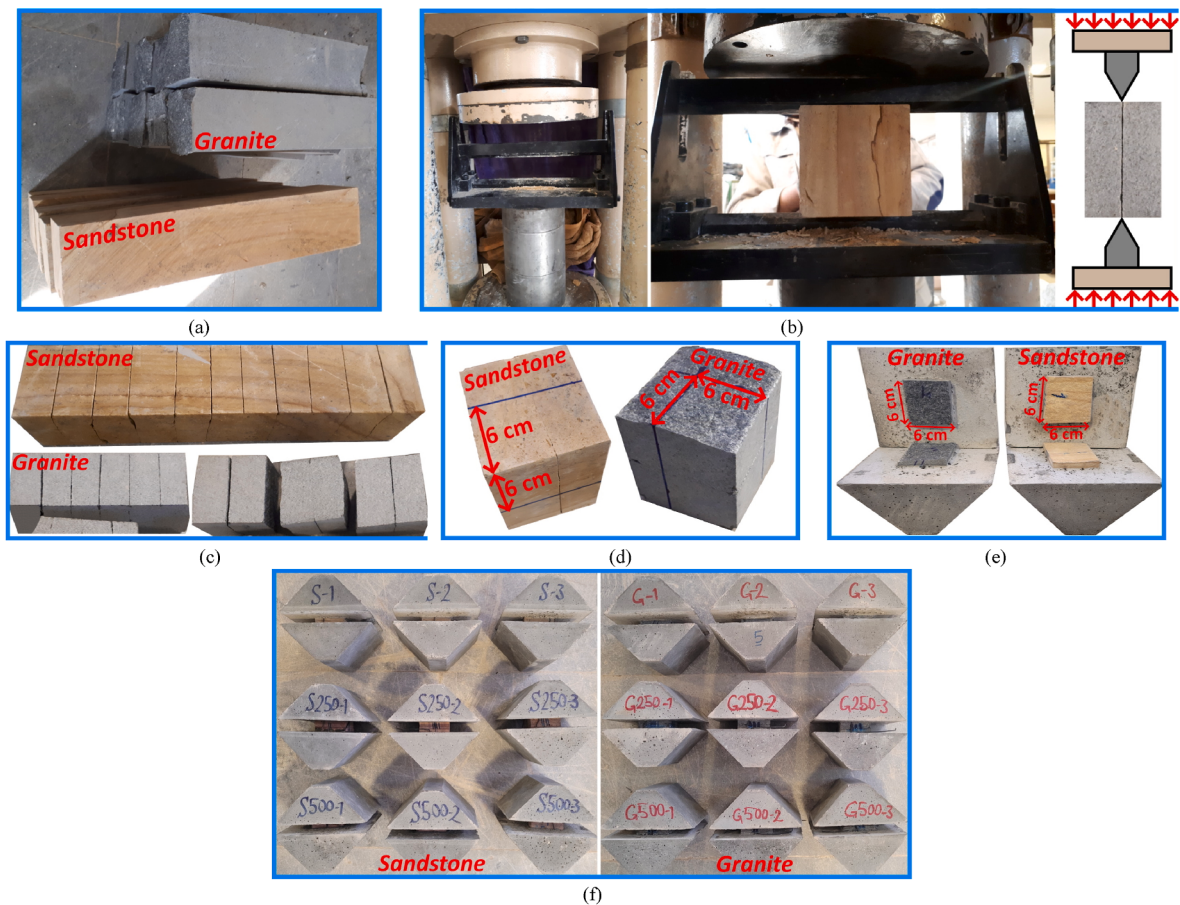
Fig. 2. Sample preparation: (a) Prismatic blocks of sandstone and granite; (b) The method used to generate artificial tensile joints; (c) The formed joints in prismatic samples; (d) Determination of the flattest 6 cm \times 6 cm area on each joint; (e) Preparation of the resulting samples in the concrete molds of the direct shear device; and (f) The final samples adopted in this study for direct shear test.
