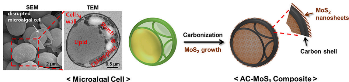
Fig. 5. Details of the carbon-MoS 2 anode composite by (Seo et al., 2019).
