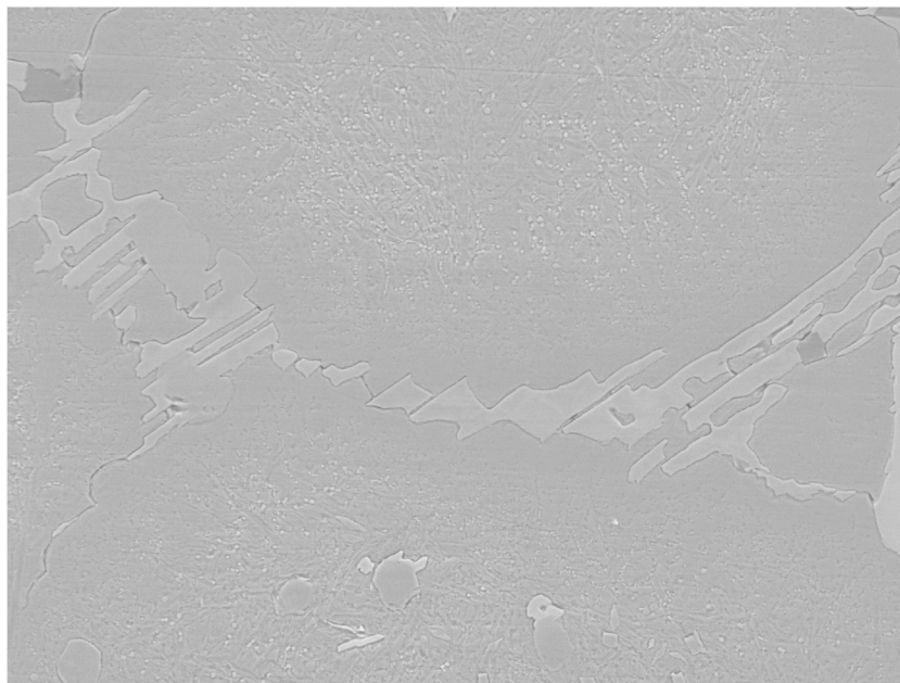
Fig. 9. SEM micrograph of sample 2 showing a cluster of M_2C lamellar morphology (light grey) and MC carbide (grey). Also evident in the microstructure MnS (dark grey) at the carbide/matrix interface.
