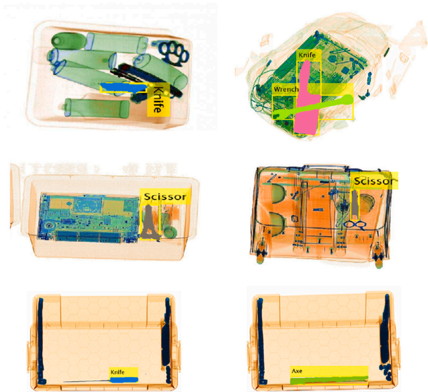
Fig. 6. Proposed framework qualitative results. The first, second, and third row represent scans from SIXray, OPIXray, and COMPASS-XP datasets, respectively.
