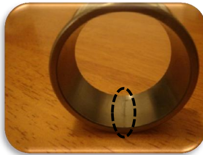
Figure 9: Pictures of faulty bearing components with line shape defect on the outer race
