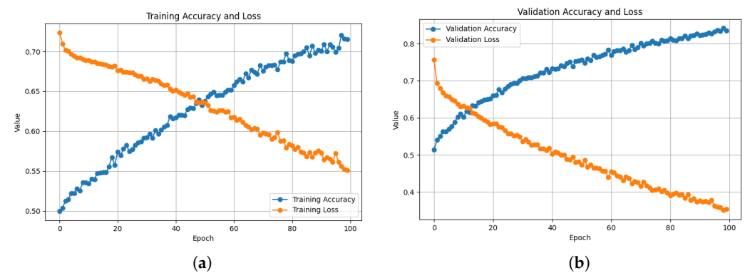
Figure 8. 1D-CNN Training and Validation Performance: Training and validation accuracy and loss curves over 100 epochs. (a) The training phase demonstrated a gradual enhancement in accuracy, reaching 85.04%, accompanied by a reduction in loss to 0.1852, signifying effective learning. (b) Validation phase demonstrating consistent accuracy improvement of 92.43% and loss reduction, indicating good generalization without significant overfitting.
