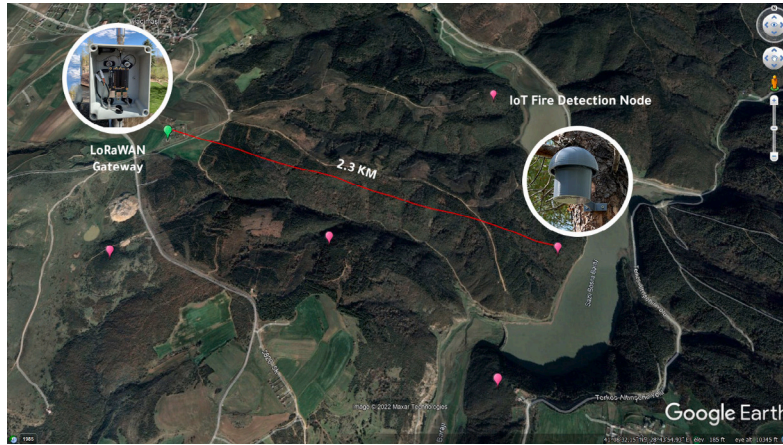
Fig. 14. The map of the forest showing the locations set for the testing nodes and gateway.
