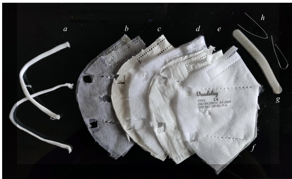
Fig. 1. Various parts and layers of an N95 respirator mask. (a) Elastic earloops, (b) Nonwoven spunbond PP layer (absorbent), (c) Nonwoven meltblown PP layer, (d) Hot air cotton filter layer, (e) Nonwoven meltblown PP layer, (f) Nonwoven spunbond PP layer, (g) Soft nose sponge, and (h) nose wire.
