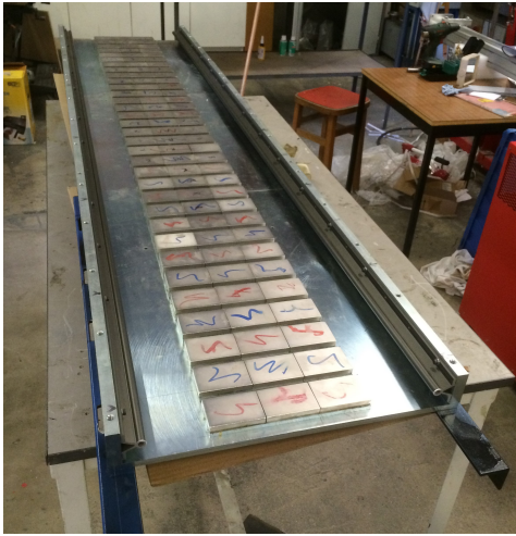
Fig. 4. Array of N45-grade NdFeB magnets placed on the steel sheet.
