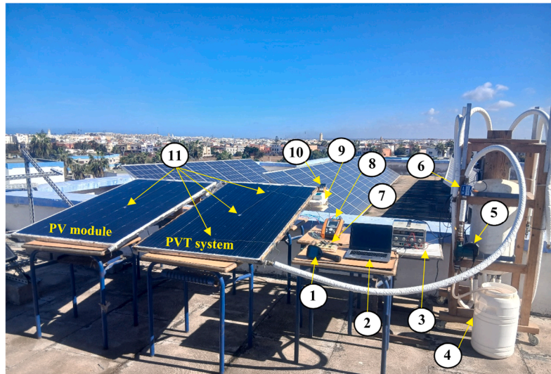
Note: (1) Infrared camera, (2) Computer, (3) Mercury thermometer, (4) Water reservoir, (5) Pump, (6) Flow meter, (7) Data acquisition and transmission system, (8) I-V tracer, (9) HT304n reference cell, (10) SOLAR -02 sensor, and (11) Thermocouples.
