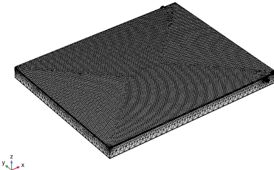
Fig. 4. PV/T collectors mesh using a user-controlled mesh sequence in COMSOL software.
