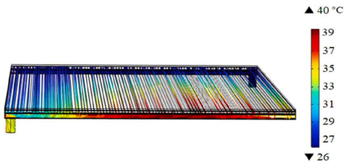
Fig. 11. Water streamlines for T_{in} and G are 26^\circ\text{C} and 10^3 \text{ W/m}^2 , respectively.
