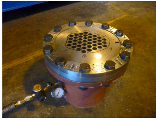
Fig. 24. Pneumatic testing of mock-up tube-to-tubesheet joint [320].
