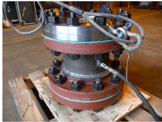
Fig. 23. Hydrostatic testing of mock-up tube-to-tubesheet for leakage [320].
