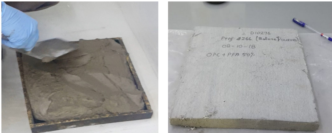
Figure 1. Thermal test specimen preparation: (a) Casting 40 X 300 X 300 mm plate for an investigated mixtures for thermal properties testing in accordance with ASTM C518-15, (b) Hardened mixture plate specimen for thermal testing.
