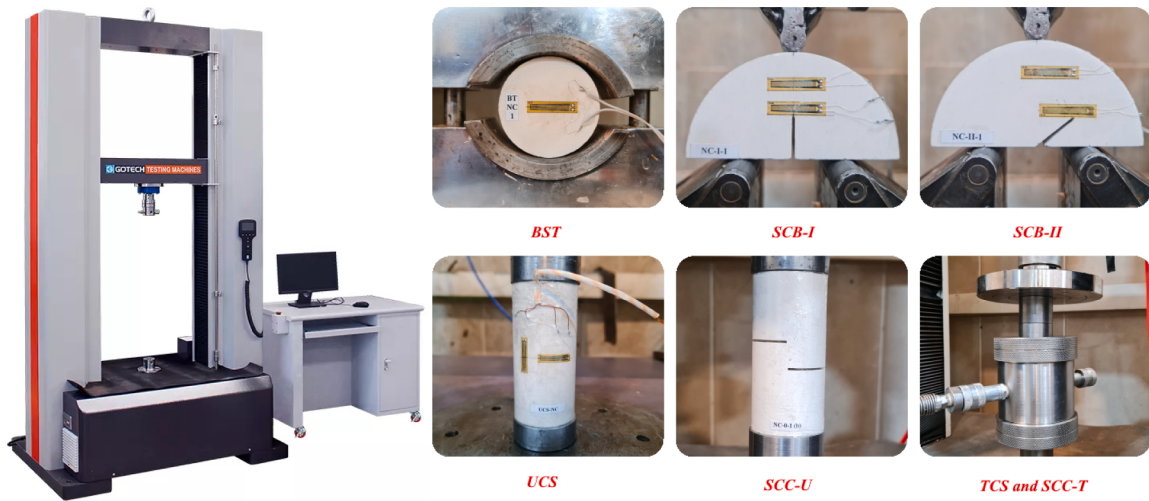
Fig. 3. Testing apparatus and loading configurations for different tests in this study.
