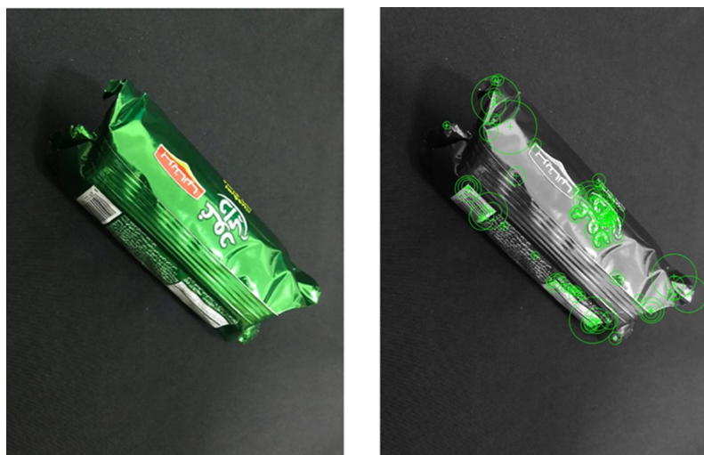
Figure 16. SURF features extracted of an item in cart.
