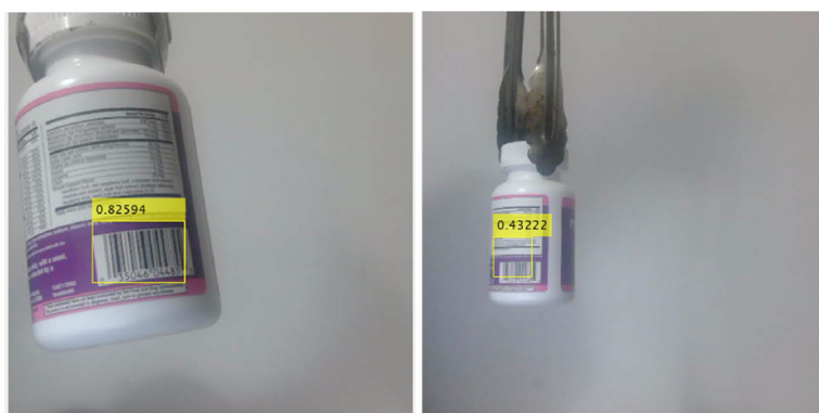
Figure 26. Detection of clear barcodes with high confidence score and unclear one with a lower confidence score.
