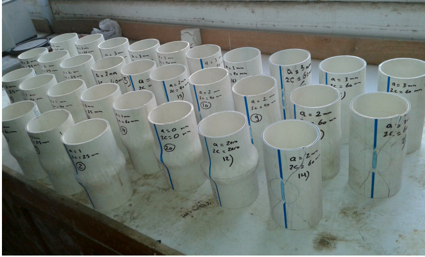
Fig. 10. Specimens after burst testing.
