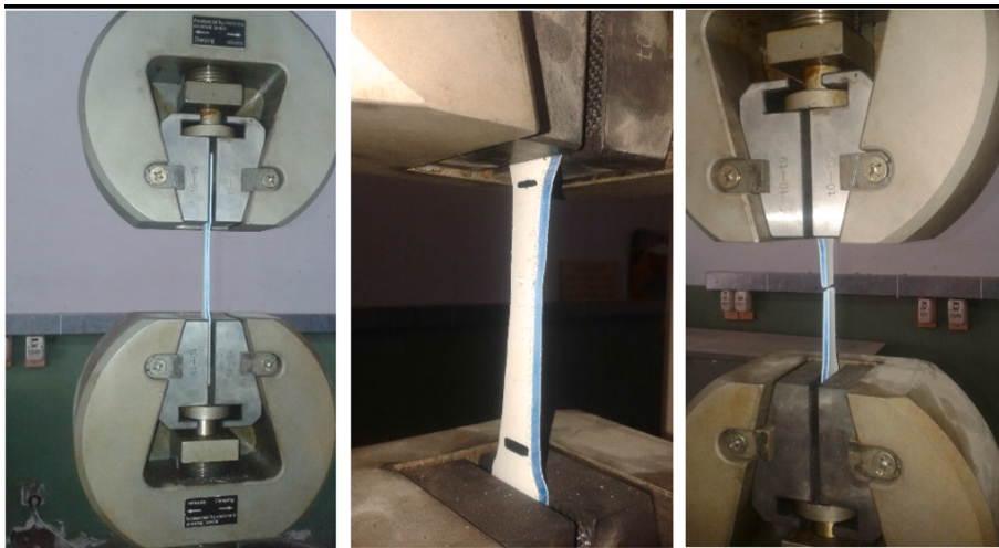
Fig. 4. The tensile sample before, while and after testing.
