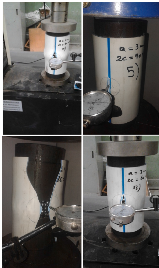
Fig. 9. Failure of cracked specimens in the burst test.
