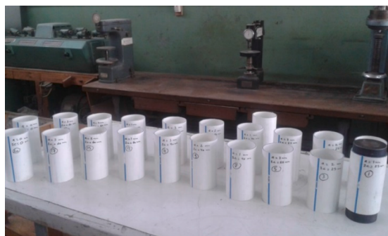
Fig. 6. Test specimens that were prepared for the burst test.
