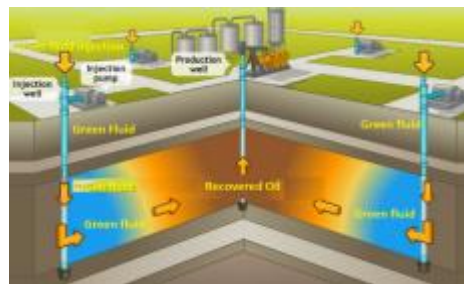
Figure 1: Schematic drawing of the injection of green water in the reservoir
