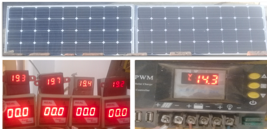
Fig. 1. Cleaned (Left) and uncleaned (Right) PV modules used in the experimental setup.
